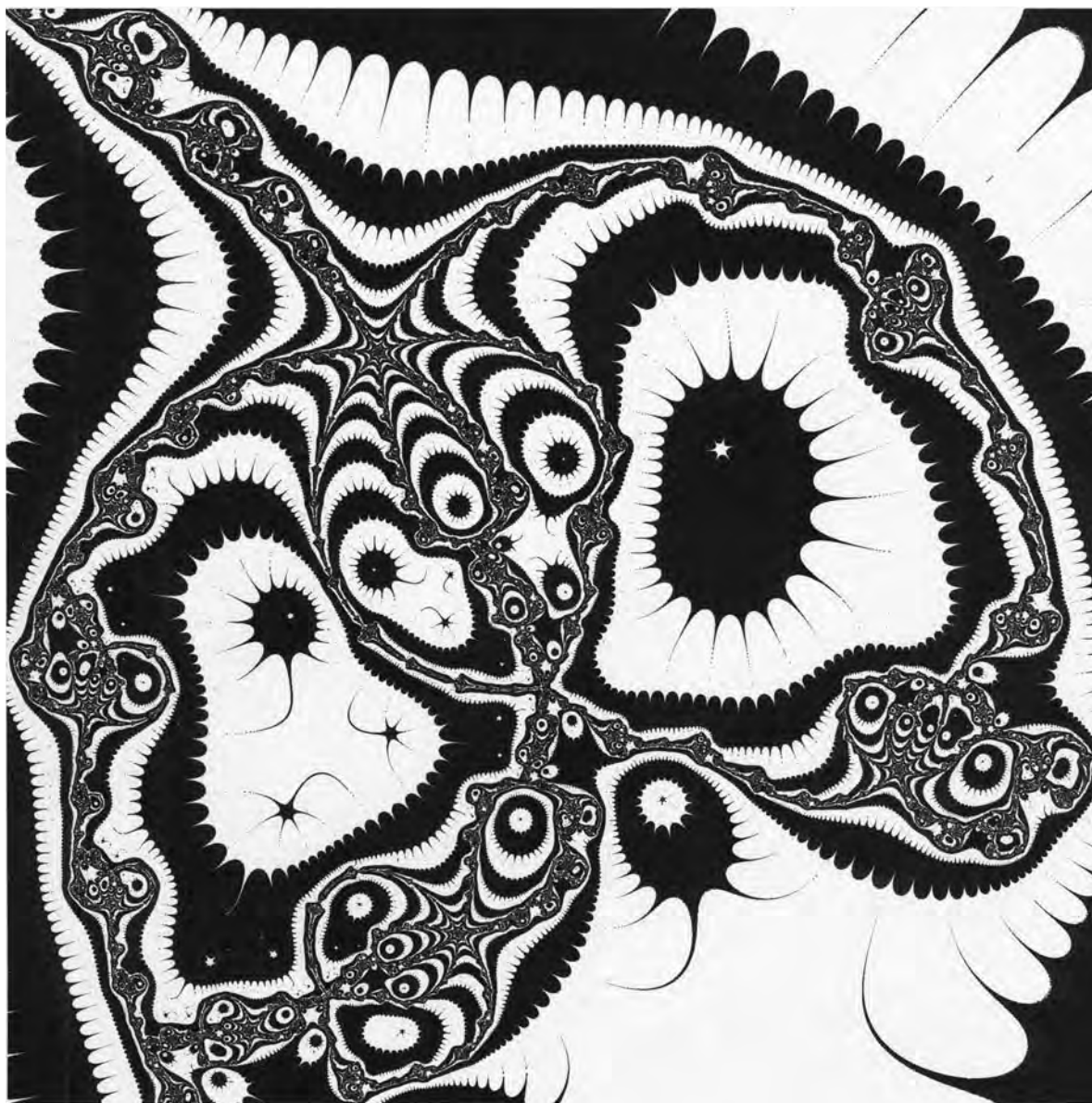
Figure 7.13 Halley map created by the author reveals the intricate behavior of a root-finding method. The problem of finding zeros of a function by iterative methods occurs frequently in science and engineering. These approximation techniques start with a guess and successively improve upon it with repetitions of similar steps. The resultant graphics give an indication of how well one of these iterative methods, Halley's method, works—where it can be relied upon and where it behaves strangely. (See pickover.com for details.)
