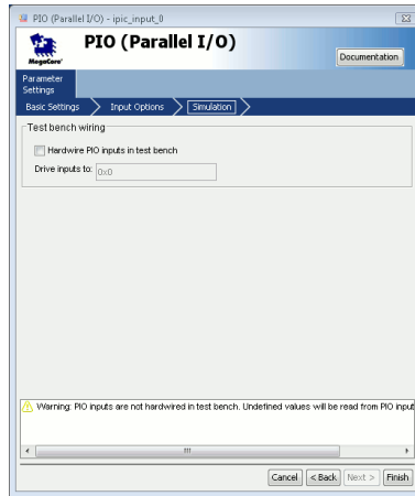
Figure 1.7: Input part of the Interprocessor Interrupt. The Figure shows the Avalon PIO simulation settings.
