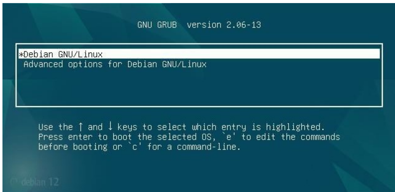
Installation: reboot on GRUB
